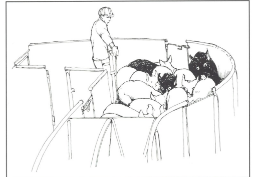
Pig crowd pen with an abrupt entrance to prevent jamming.
